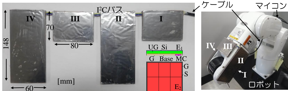
E 1 , E 2 : Electrodes, UG: Urethane gel, Si: Silicone sheet, S: Shield, G: GND, MC: Measurement circuit (AD7147 etc.)
